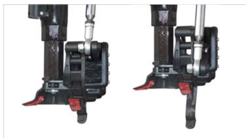
Integrated demounting lever for demounting without tyre lever.
